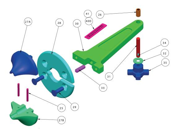
SI Hand Guards are an improvement to safety on location. If elected, SI Hand Guards can be installed on the SI 14" & 18" Top Rigging Sheave. The shield arms are set so that the taut wireline is centered in the hand shield ring and locked securely in position. The split plastic shells close around the wireline and twist-lock into the hand shield rings. These shields are sturdy, providing maximum protection. All details are universal to the left-hand and right-hand shields.
