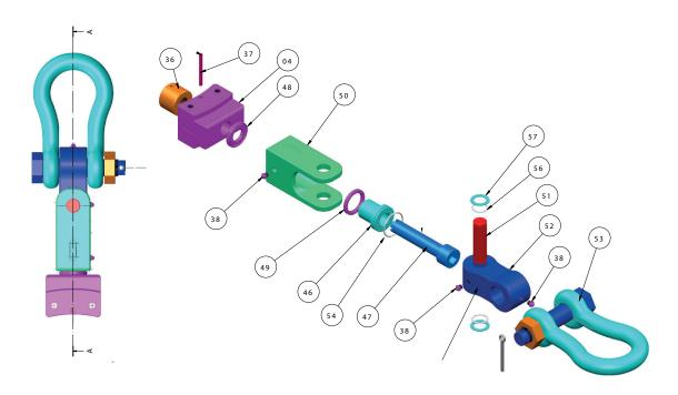
The SI Clevis Swivel improves the overhead safety as the hanging position for the SI Top Rigging Sheave can never be caught in a bind. The SI Clevis Swivel flexes bidirectional and rotates 360°.
